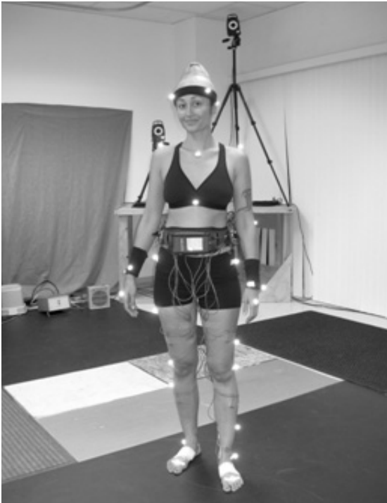
FIGURE 1. Participant with 35 spherical markers using a Plug-in Gait Full Body Marker set.
